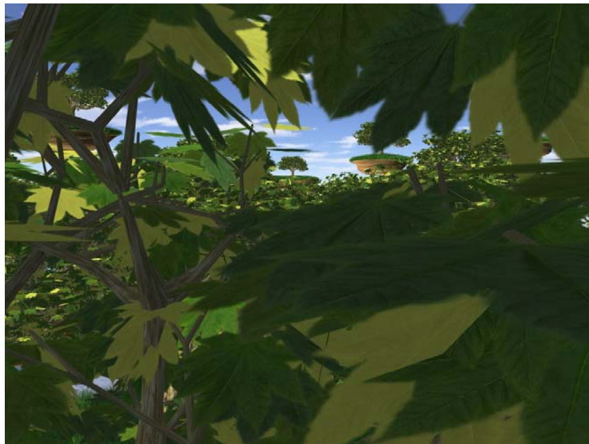
Figure 9. Using alpha to coverage, leaf edges in alpha textures receive the smoothing effects of anti-aliasing.
